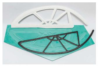
Spickenheuer's team has since employed a similar five-step design process to redesign and replace two aluminum attachments for the rear wing of a racecar, using variable-axial CFRP.
